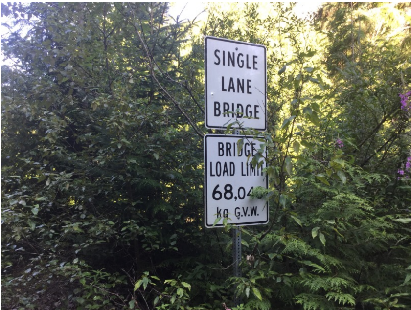
Load Posting Sign
